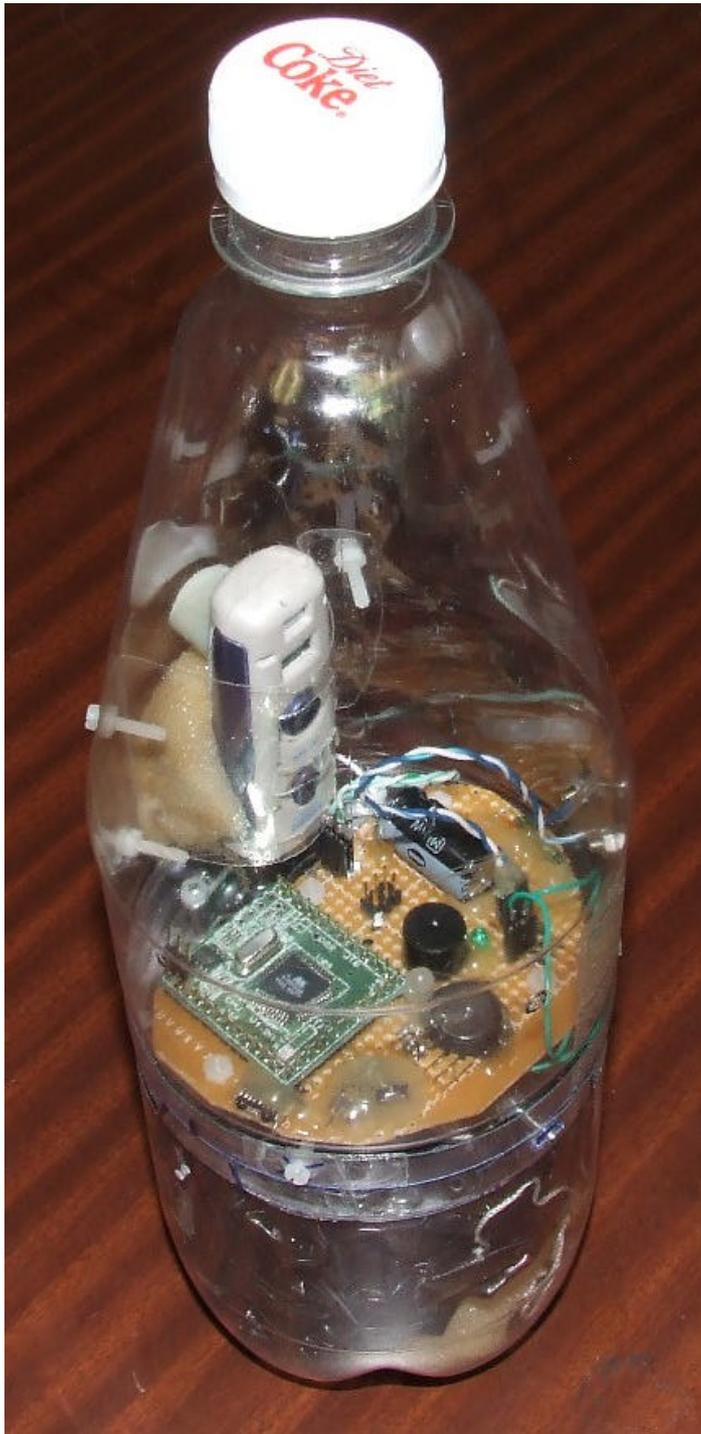
The complete H2O Rocket Controller in the nose-cone, atop the parachute compartment. All ready for installation onto the rocket body.
